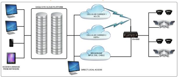
**Cloud or Local:** The Eagle Eye platform allows you to record to the cloud for small installations and record to a local cloud-managed NVR for larger installations
