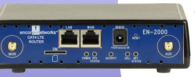
The Encore Networks EN-2000™ is a high performance ultralow cost M2M VPN network router designed for the Verizon Wireless LTE public and private networks. Ideally suited for the 'Internet of Things,' this compact IP M2M router provides license free IP, VPN, Firewall, Ethernet and IP interworking with an embedded Verizon LTE cell module and an integral Wi-Fi access point for 802.11n at 5 GHz. Servicing the needs of mission critical business and enterprise applications
