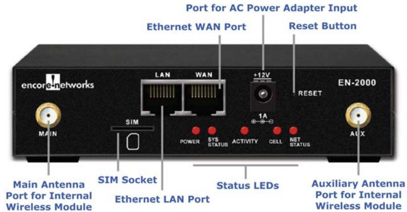
The EN-2000's WAN port (also on the rear panel) is on a separate network from its LAN port. The EN-2000's WAN port is a DHCP client, by default.
