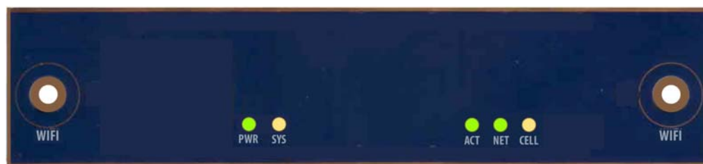
Figure 1-4. EN-2000 Back Panel without Serial Port LEDs
